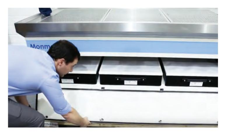
When servicing/calibrating/validating it is important to check all aspects of a cabinet. Monmouth Scientific utilise the latest equipment (Vane Anemometers, Particle Counters, Smoke Generators & Photometers) to carry out:
